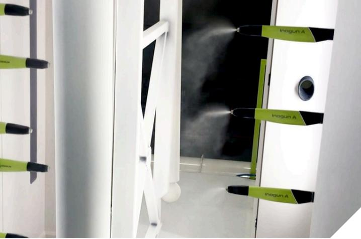
The **Inogun range** is built upon a common base, thoroughly tested, and available with different fixing gear according to needs in the powder booth: the **Inogun A** rear fitted flange to be tilted towards the parts and the **Inogun A FCC** (Fast Color Change) with its smooth droplet shape for easy color changes.
